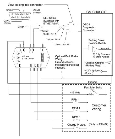
PTO output is +12 volts at 3 amps and is set when the throttle control is actively controlling the engine rpm and the Chassis Ready Conditions are satisfied. Do not connect any +12 volt sources to this output terminal or damage may result voiding the warranty.
