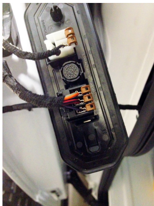
Figure 5. View of Side Door Ajar switch
