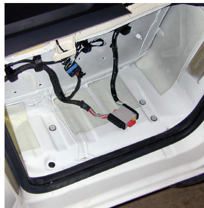
Figure 6. View of stepwell wiring and potential splice site.
