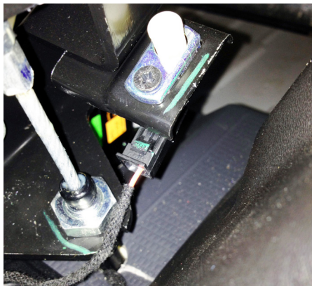
Figure 4. View of Park Brake terminals
