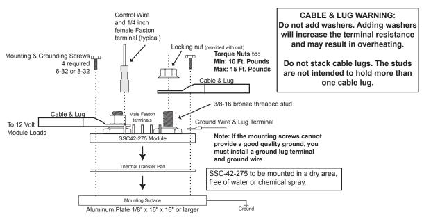
Note: The Mounting Surface provides a means to remove heat generated by the SSC42-275. If this surface is a poor conductor of heat, the disconnect switch will have a lower current rating than if the surface is a good conductor
