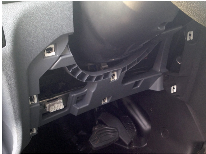
Figure 2. Steering column with panel removed.
