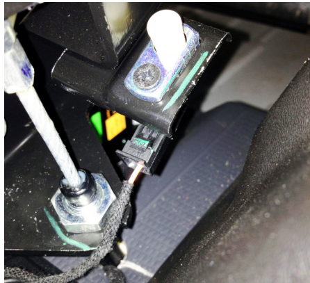
Figure 4. View of Park Brake terminals
