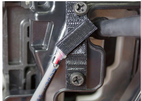
Figure 3. View of proper placement of sensor beside the shifter shaft.
