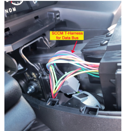
Figure 5. SCCM Connector T-Harness Data Bus
