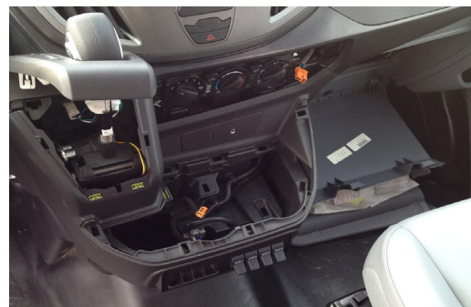
Figure 7. Removed to Access Shift Lock Connector
